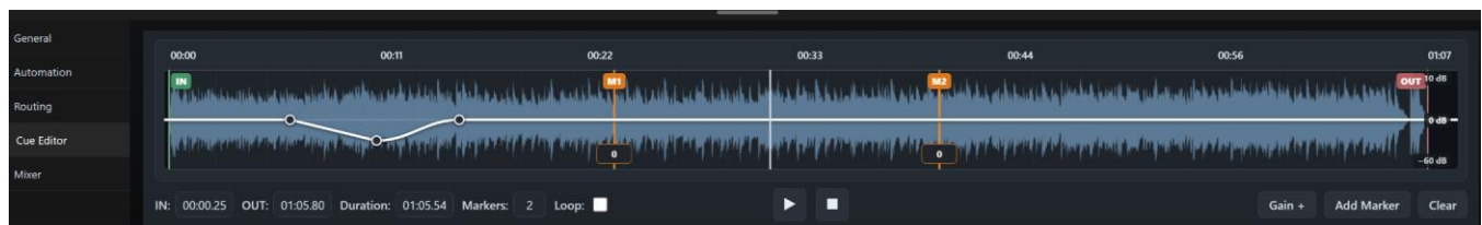
Audio Cue Editor with waveform, IN/OUT, gain envelope and markers.
